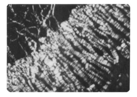
Figure II. A photomicrograph of a concentration gradient set up by running  $\text{D}_2\text{O}$  against a 30% CsPFO lamellar sample. Temperature 20°C. The right lower corner has the highest  $D_2O$  concentration.
